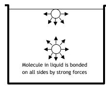
The study and engineering of fluids where surface tension dominates (usually in thin tubes or channels) is called *microfluidics*. In many circumstances (like large pipes or external flows) we can ignore the effects of surface tension.
