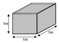
This amount of water would weigh 998Kg. Therefore we say that water has a *density* of 998 Kg m<sup>-3</sup>. Some other important densities are: Paraffin - 800 Kg m<sup>-3</sup> (because it's less dense that water, it will sit on top) and Mineral Oil (the type which lubricates your car) - 880 to 950 Kg m<sup>-3</sup>.
