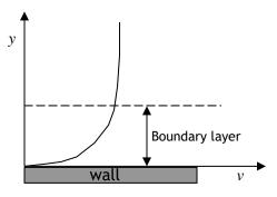
The (sometimes thin) layer where the fluid speeds up is called the boundary layer and although it may be small it can have an important effect on the system.
